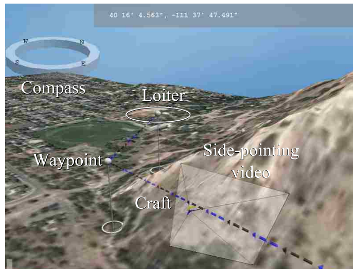
Figure 4.22: Full 3D interface—following waypoints
